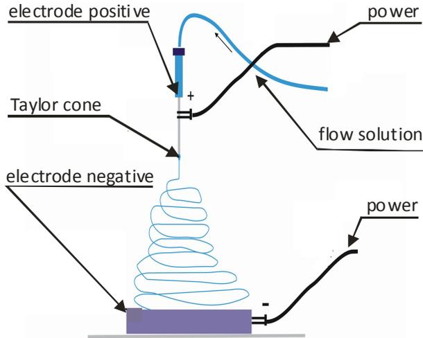
**Figure 2.7.** Nanofibers electrospinning schematic
