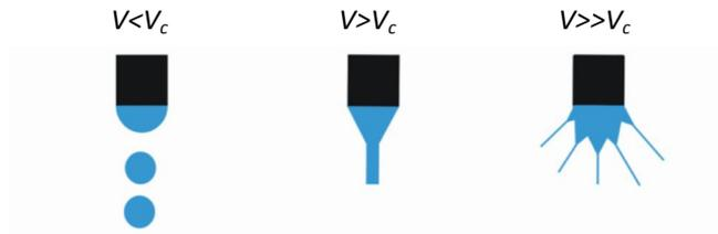
**Figure 2.9.** Influence of electrostatic field on solution
