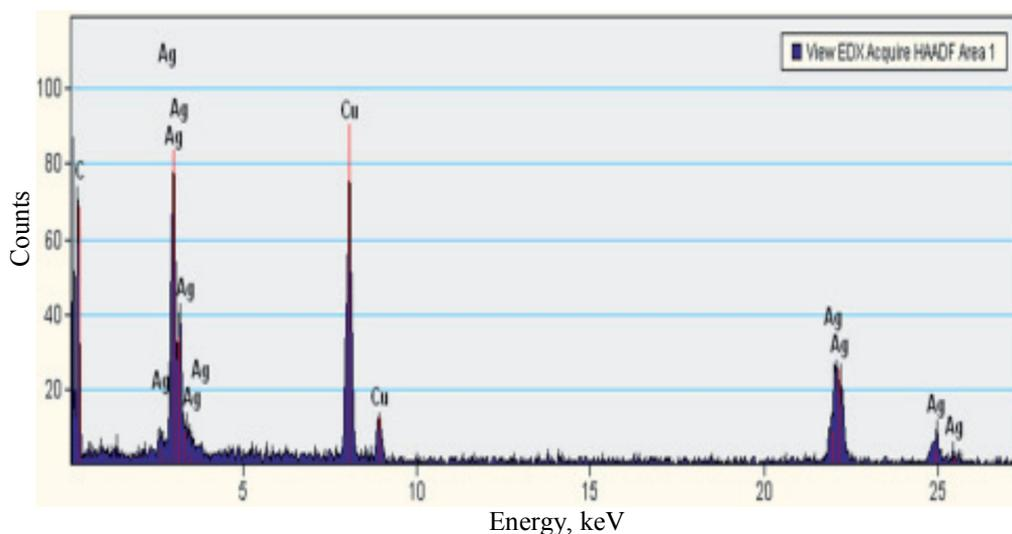
**Figure 2.14.** The example of using EDX technique for the investigations of the composite nanofibres containing silver on the surface; peaks for copper derive from the copper support mesh applied
