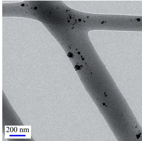
**Figure 2.15.** The example of using high-resolution transmission electron microscope HRTEM for the investigations of the structure of obtained composite fibres with 5% addition of silver nitrate; a photograph taken after precipitation of silver with a 2% ascorbic acid solution
