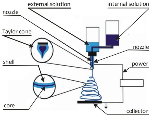
**Figure 2.10.** Simplified co-axial electrospinning
