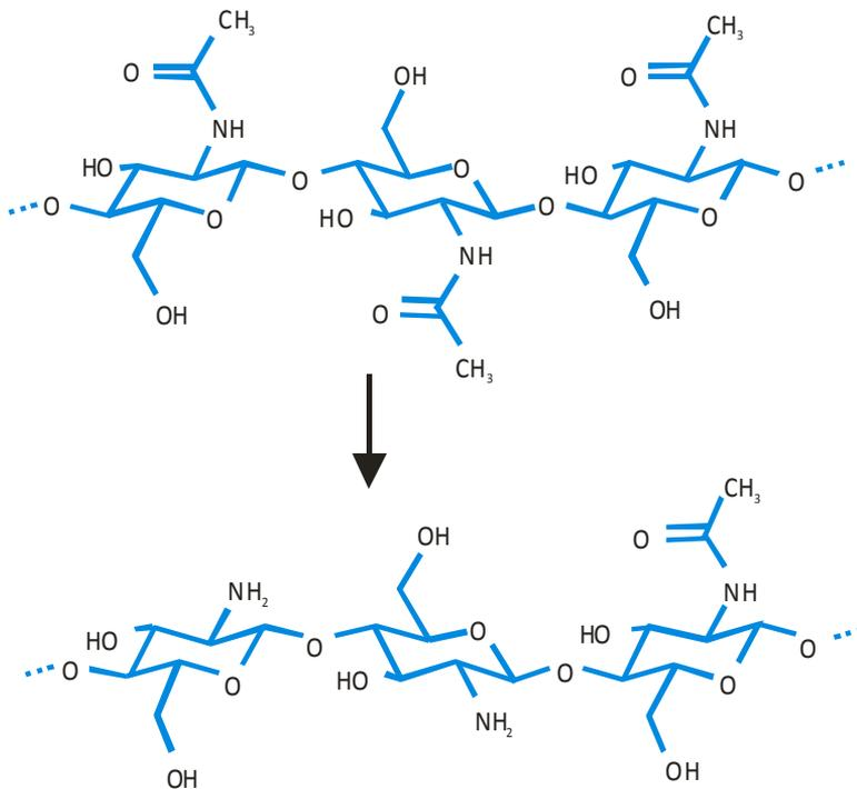
**Figure 2.1.** Structure of chitin and chitosan macroparticles
