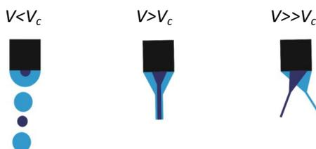
**Figure 2.12.** Electrostatic field acting on the stream of polymer solution;  $V < V_c$  – field below critical value;  $V > V_c$  – optimum field;  $V \gg V_c$  – supercritical field
