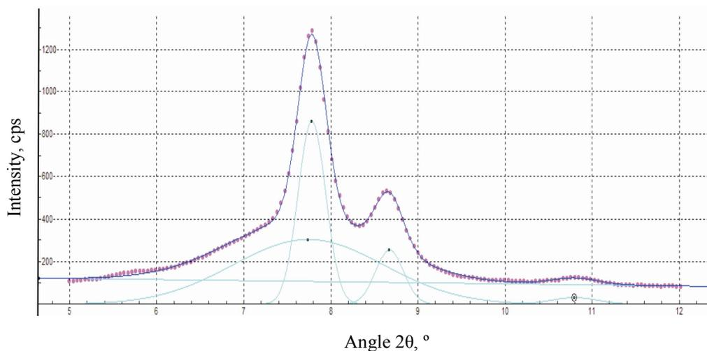
**Figure 2.17.** The example of using the Wide-angle X-ray scattering WAXS technique with approximation of radial profiles, determination of the degree of crystallinity based on Levenberg-Marquart method for polycaprolactone fibres deposited onto the rotational collector with the rotation speed 500 rev./min
