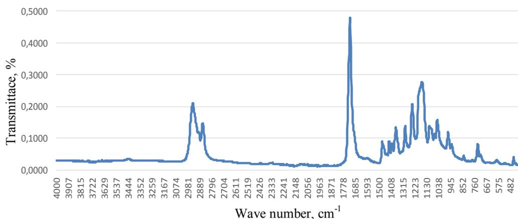
**Figure 2.18.** The example of using the FTIR method for the investigations of obtained polycaprolactone fibres from a 10% solution in a mixture of formic acid and acetic acid of 70:30 m/m deposited onto the rotational collector with the rotation speed 500 rev./min
