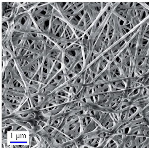
*Figure 2.13. The example of using SEM technique for the investigations of the morphology of obtained polycaprolactone fibres from a 10% solution in a mixture of formic acid and acetic acid of 70:30 m/m*
