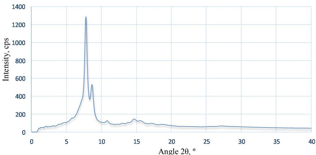
**Figure 2.16.** The example of using the XRD analysis of the phase composition for the investigations of the polycaprolactone nanofibres obtained using a rotational collector
