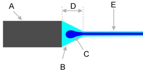
**Figure 2.11.** Co-axial core consists of, A – jet responsible for jacket formation, B – solution of external jet, C – second external jet situated in the place where the Taylor cone is formed, D – Taylor cone of internal solution, E – co-axial nanofibers
