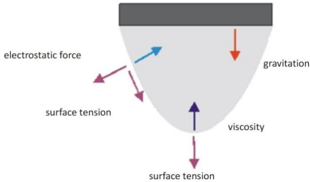
**Figure 2.8.** Electrostatic forces acting on a droplet of polymer solution
