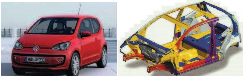
Figure 6.4. Monobloc automotive “body in white” structure. Colour-marked elements are made of stamped steel sheets: red: advanced ultra-high strength, yellow: very high strength steel, blue: - High strength steel, light blue – steel parts prone to absorb impact energy, purple - hot-stamped steel sheet
